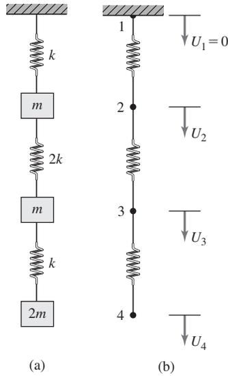
**Figure 10.6** System with 3 degrees of freedom for Example 10.3.
