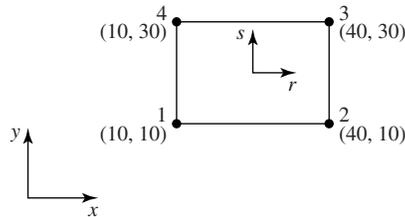
**Figure 10.12** The rectangular element of Example 10.6.
