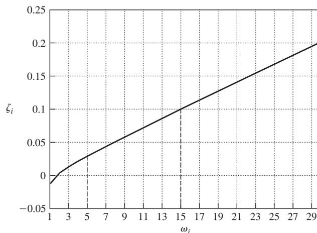
**Figure 10.16** Equivalent damping factor versus frequency for Example 10.9.
