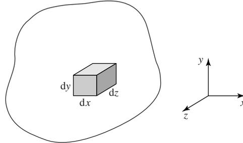
**Figure 10.11** Differential element of a general three-dimensional body.
